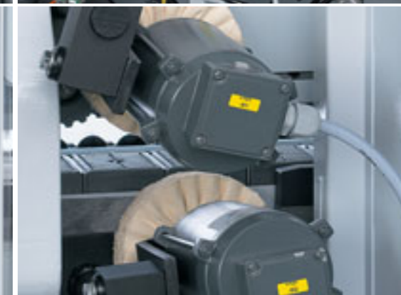
Buffing unit Buffing unit to polish edges and maintain their natural colour.
