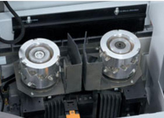
Joint trimming unit Perfect cut and high operating life due to diamond tipped tools for an optimum edge joint quality.
