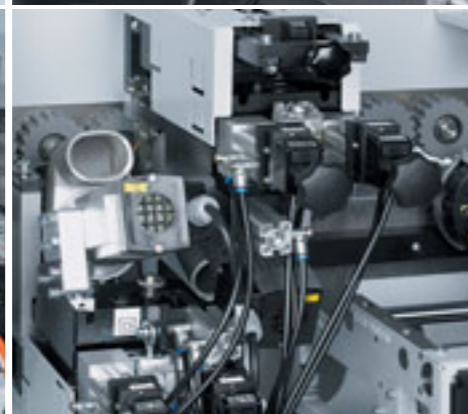
Trimming unit with pneumatic 3-point adjustment (optional) For even more effective production and much shorter changeover time.
