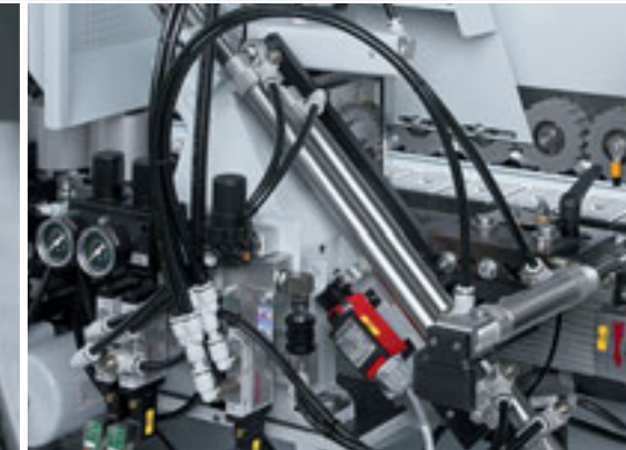
End-trim unit Precise end-cut through a strong end-trimming unit, equipped with THK guides. Chamfer/straight adjustment by easily tilting the unit. (Pneumatic adjustment optional)
