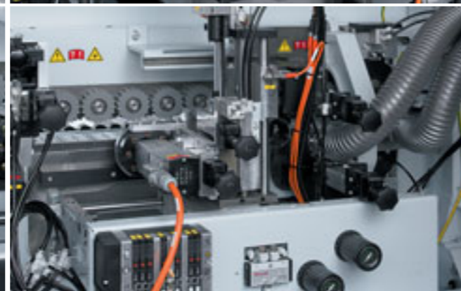
Corner rounding unit Optimum corner rounding without adjustment or set-up, resulting from the coupled diamond tool and tracer roller. Workpiece thickness up to 40 mm.
