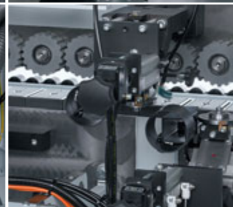
Profile scraping unit Unit to smooth radii or chamfers, equipped with quick change heads for fast profile change (Pneumatic adjustment optional).
