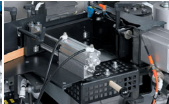
Gluing unit and magazine Coil and automatic strip magazine for a reliable edge material supply. Optimal glue joints, by controlling the exact amount of glue.
