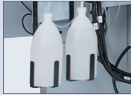
Spraying unit (optional) Separation and detergent agents for a perfect finish when processing PU-glue.
