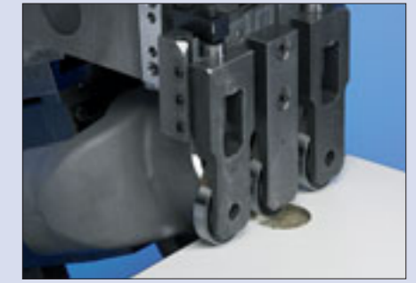
Nesting package (optional) Includes a multi-roller tracing device for the trimming and scraping units to compensate for hinge holes.
